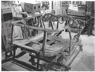
Top photos show two views of the ash framework assembled to the newly powdercoated chassis.
