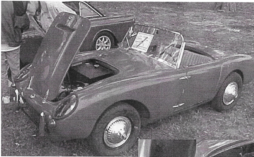
Left: Charles Vestweber's 1958 Berkeley B65. Motorcycle engine, below, barely larger than the battery, powers tiny car.
