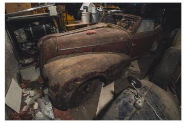
company's standards in an abortive attempt to stave off the Liquidator. The upholstery is rotten, woodworm has almost finished its meal on the ash frame, and the fenders are full of rust holes. There are no headlights or instruments.
