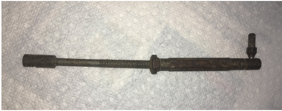
Part of the carburettor linkage for an SU on many British cars.
