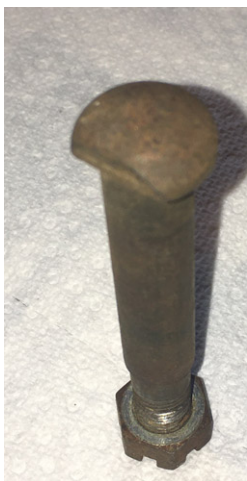
Shown, above is a fulcrum or trunnion bolt that holds an MGB front shock absorber to the swivel axle.
