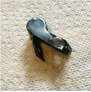
This is a 'finisher' for the rubber seal for the door opening in an MGB.
