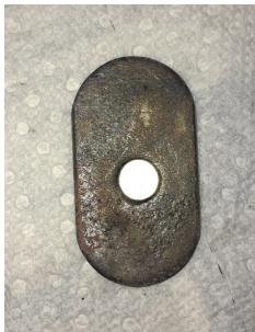
Part of the carburettor linkage for an SU on many British cars.
