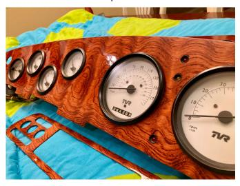
Once I swapped all the gauges over from the old fascia, I changed all the illumination to LED and installed new switches for the lights and flashers. I also glued new Plexiglas to the underside, creating lenses over the warning and turn signal indicators.
