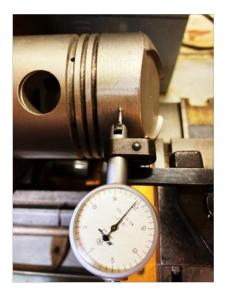
same function, but smaller and perhaps not as fine quality. For demonstration purposes, I've chucked up an old piston in my lathe and clamped the dial indicator for measuring eccentricity. This style is smaller and better in small spaces, but lacks its own clamp.
