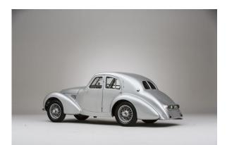
rectangular steel tubes, which varied in both dimension and thickness based upon anticipated stresses. To add rigidity, a second rectangular tube space frame, this one intended to support the car's aluminum body, was welded to the car's chassis, creating a light yet strong platform from which to build a grand touring car. Underneath, Aston Martin the automaker's firstever independent front suspension, while keeping a live axle and traditional leaf springs in the rear.
