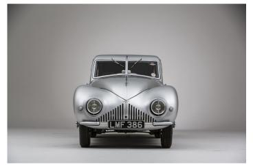
the Atom had fenders that flowed into the body eliminating the need for running boards. The Atom's headlamps recessed into the front fenders for a cleaner look and improved airflow. The car lacked any grille to speak of, Instead, a series of 12 slits, tall in the center then each smaller moving outward. Wartime material shortages may have influenced the car's lines, but it's clear that Hill and Sutherland always
