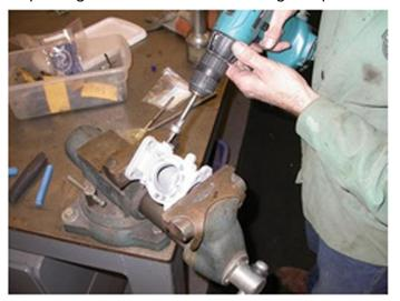
reaming out the old bushings, installing new bushings, and reaming the new bushings to size.
